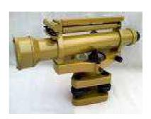
8) Tilting Level: It is used for taking invert staff reading
