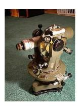
16)Tacheometer: It is nothing but transit theodolite fitted with the stadia diaphram and an analytic lens.
