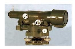
9) Auto-level: auto level is used for taking the reading from the long distance and its best part is it is automatic leveled.
